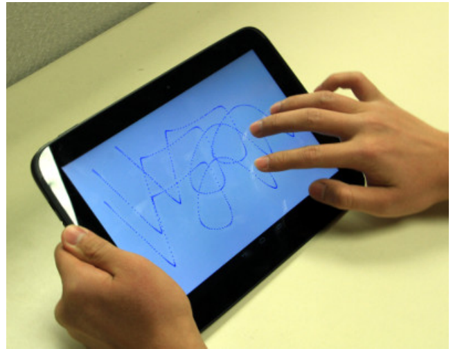
Figure 1: This paper studies continuous free-form multitouch gestures as means of authentication on touchscreen devices. Authentication on touchscreens is normally done with a grid-based method. Free-form gesture passwords have a larger password space and are possibly less vulnerable to shoulder surfing. We note that there are no visual cues for the gestures, the gesture traces are shown only after creating the gesture.
